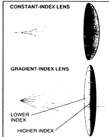
**GRADIENT-INDEX LENSES** can correct for spherical and other optical aberrations by continuously changing the refractive index (bottom). Light rays hitting a conventional lens, with its single refractive index (top), may fail to reach a single focal point. Isotec's gradient-index glasses (photograph), which are being developed into lenses, can bend light independent of wavelength or surface curvature.
